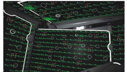
Points measured in 3D and recognized by V-STARS (photo library: Airbus).
