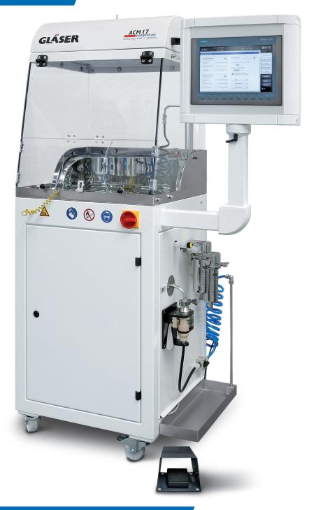
Extraction system in the second generation. Latest state-of-the-art technology for the inspection of Technical Cleanliness on functionally relevant components. Re-engineered in accordance with the recommendations of VDA 19.1 chapter 11 for work safety and protection of the environment. The ACM17 is perfectly suitable for your requirements in future.
