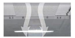
SUPPLYING of filtered air passes over the flow cap top. Active protection of components and the flushing bowl against contamination. This produces an ISO 5-class like extraction area. High occuptional safety by connecting your extraction to our cabinet.
