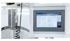
12" BASIC TOUCHSCREEN with intuitively operable software. Simple operating due to password-secured user-levels and the possibility to save test processes. Continuous monitoring of safety relevant functions. Optional comfort touch panel with separate keyboard with easy to clean glass surface available.
