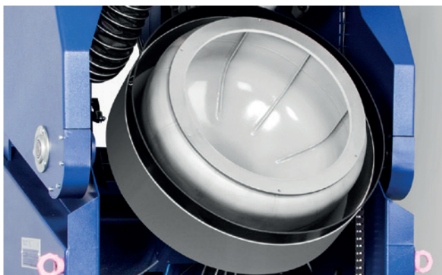
Drum with 3S lining
