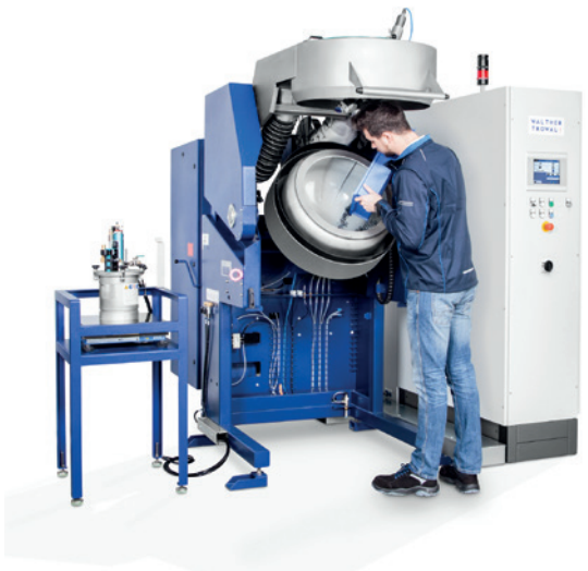
Loading of the drum with uncoated work pieces
